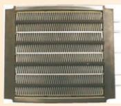
PTC finned resistor heaters are dynamic heating elements designed to heat up moving air. The large surface area of the aluminum fins ensures a homogeneous heat transfer adjusting the air volume flow. This system allows an automatic regulation of the heating power within certain ranges. Due to the features, there are many application possibilities. In addition to the standard types, special versions for specific applications are available.
