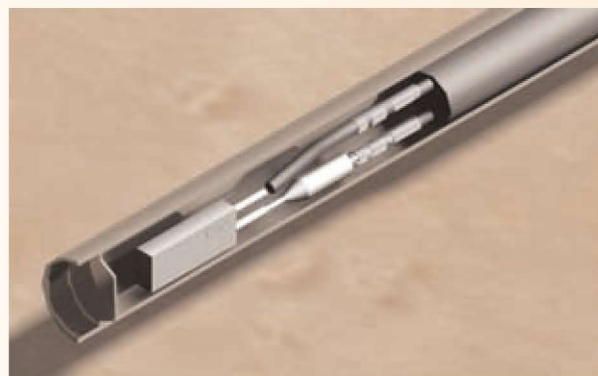
Detail of implementation of the thermostat and safety fuse in a Class II single tube heating element for towel rails.
