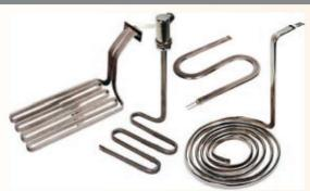
RKF flat tubular elements have a wide range of applications. Its oval-shaped cross-section is particularly adapted to contact heating. The larger contact surface area of these resistors compared to round-tube resistors enables production of shorter resistors with higher load densities.
