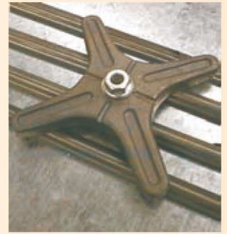
Example of installation with 4 L-ETM heating element with cross bridle
