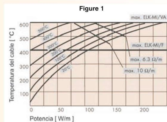
Generally, maximum working temperature is known (in the piping or superficial temperature). The intersection with the working temperature curves shows us the relationship between the maximum temperature of the lead (vertical) and its maximum lineal power (horizontal).
