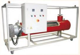
GCP pass superheaters consist of a GCB heating group assembled on a steel or stainless steel tubular body, of suitable flange, bed and entry, exit and purge tubulatures, threaded or flanged. The fluid to be heater circulates inside the same, guided by the deflectors at intervals in the heating group.
