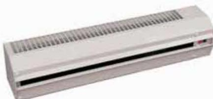
**Description:** Hot air curtains fitted with a tangential fan. Solid painted steel chassis. Fitted with a selector switch for stop, ventilation and heating. Protection level IP31.
